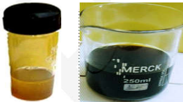
Fig. 1: The mixture of plant leaf extract and \text{AgNO}_3 solution i. At the beginning ii. After 5 hrs
